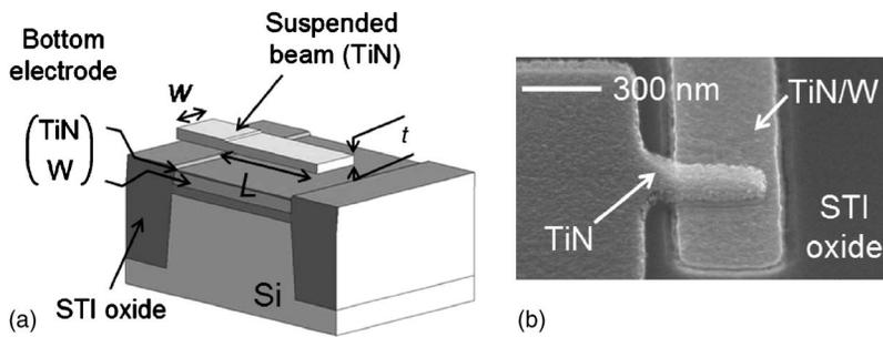
FIG. 1. (a) Schematic diagram of the cantilever-type NEM switch composed of the suspended beam and the bottom electrode. (b) SEM photograph of the cantilever-type NEM switch fabricated by using conventional top-down CMOS fabrication technology.
