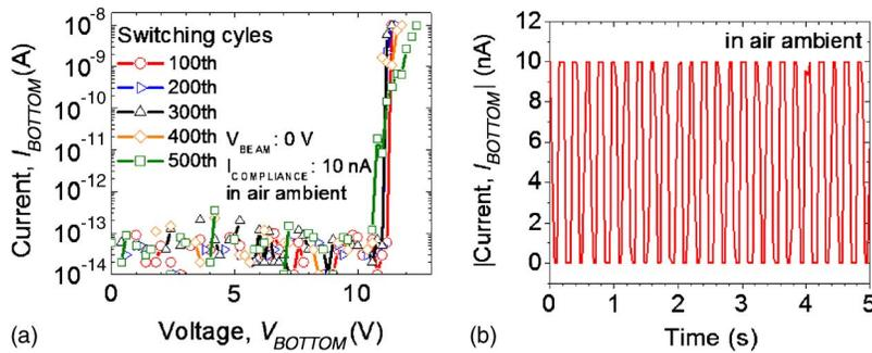
FIG. 4. (Color online) (a)  $I$ - $V$  plot of the fabricated cantilever-type NEM switch ( $w/L/t = 200$  nm/300 nm/35 nm) under dc bias in air ambient. (b) The output current of the cantilever-type NEM switch ( $w/L/t = 200$  nm/300 nm/35 nm) as a function of time under ac bias in air ambient. Note that an ac bias with a peak voltage of 15 V and a square wave of 5 Hz were applied to the bottom electrode.
