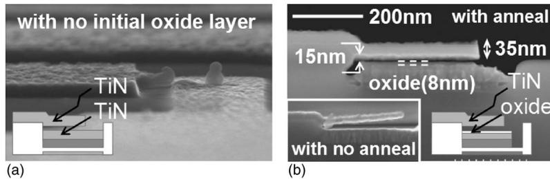
FIG. 2. SEM photographs of (a) the disappeared beam by the localized contact melting, which has no initial oxide layer and (b) the successfully fabricated and flat cantilever-type NEM switch by employing an ultrathin oxide layer and an annealing process. The inset shows the suspended beam fabricated with initial oxide layer and no annealing process.
