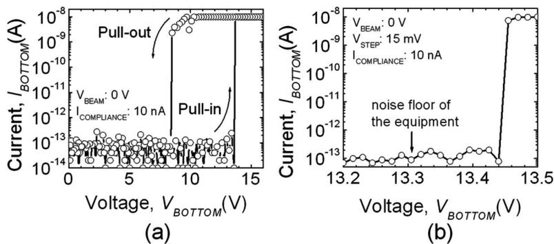
FIG. 3. (a)  $I$ - $V$  hysteresis curve of the fabricated cantilever-type NEM switch ( $w/L/t = 200 \text{ nm}/300 \text{ nm}/35 \text{ nm}$ ). (b) Magnified view of the pull-in region, showing ideal on/off current characteristics.
