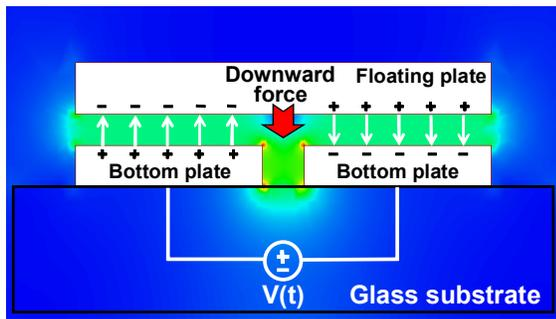
Figure 2. Electrostatic field simulation result performed by Maxwell<sup>®</sup> 2D showing E-field confinement between two fixed bottom plates and the electrically floating top plate.
