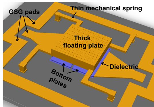
Figure 3. Actual structure design of the proposed variable capacitor.
