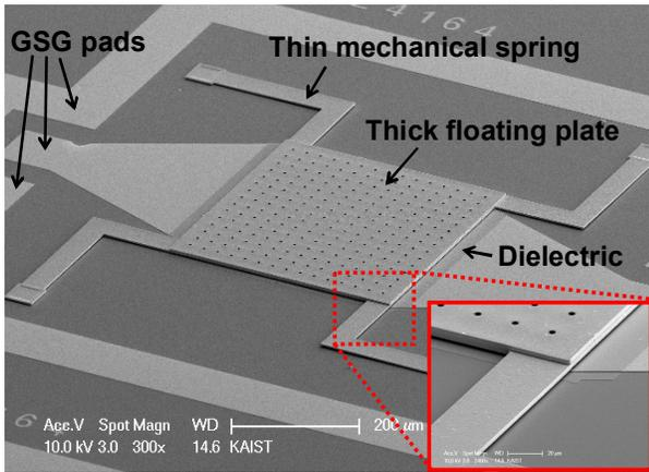
Figure 5. SEM photograph of the fabricated variable capacitor.
