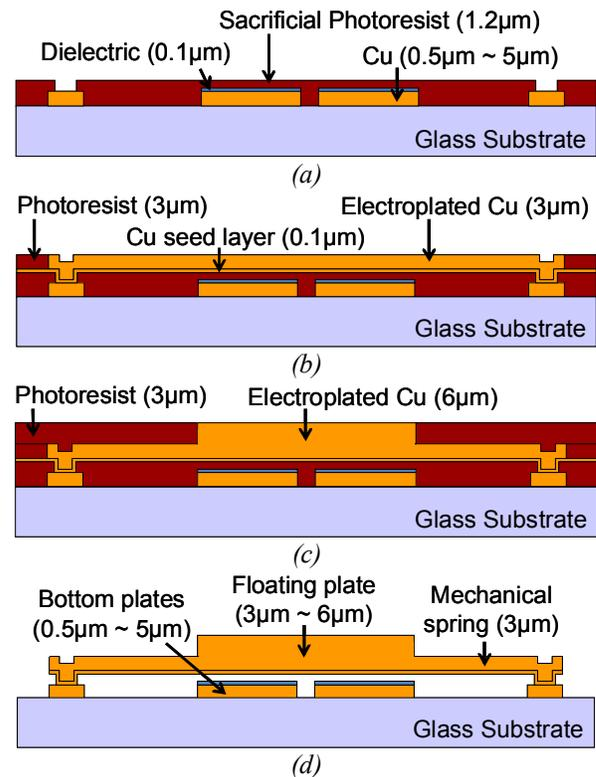
Figure 4. Simplified fabrication process (a) Deposition and patterning of the bottom plate, dielectric, and sacrificial photoresist (b) Cu seed metal deposition and patterning of the thick photoresist followed by Cu electroplating of the floating plate and mechanical spring (c) (Optional) Patterning of the thick photoresist and Cu electroplating of only the floating plate area (d) Releasing by sacrificial layer etching.
