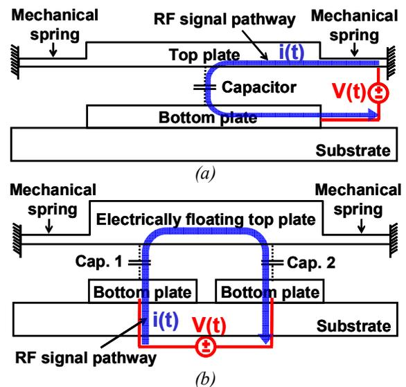
Figure 1. A schematic view of (a) conventional variable capacitor with two parallel-plates (b) proposed variable capacitor actuated with an electrically floating top plate.
