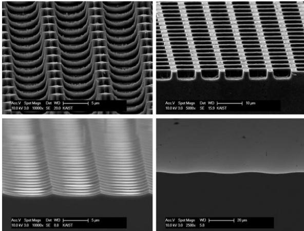
Figure 6. SEM images of various shapes or slopes of 3-D silicon microstructures.
