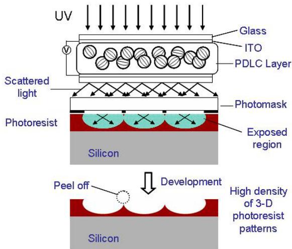
Figure 2. Schematic views showing the fabrication principles for a high density of 3-D photoresist microstructures by 3-D lithography using PDLC films.
