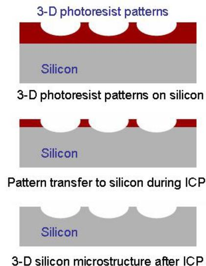
Figure 3. Process flows of pattern transfer to silicon using ICP etching process.
