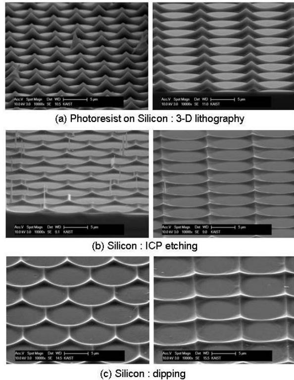
Figure 5. SEM images of (a) 3-D photoresist microstructures on a silicon substrate by 3-D lithography, (b) 3-D silicon microstructures by ICP etching process, and (c) 3-D silicon microstructures by dipping process with wet-etchant.
