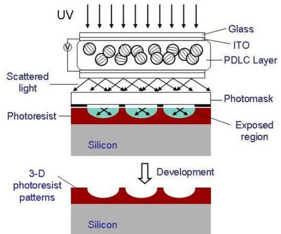
Figure 1. Schematic views showing the fabrication principles for 3-D photoresist microstructures by 3-D lithography using polymer dispersed liquid crystal (PDLC) films.
