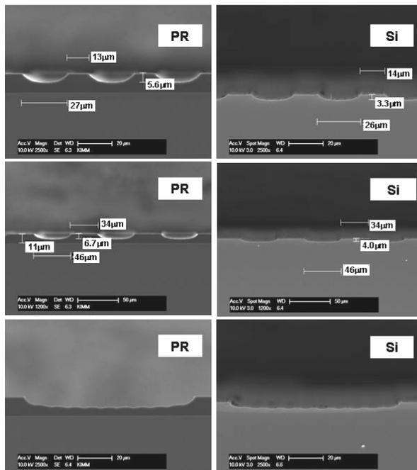
Figure 4. SEM images of cross-sections of 3-D photoresist microstructures with various sloping profiles acquired by 3-D lithography (left figures) and 3-D silicon microstructures transferred by ICP etching (right figures).
