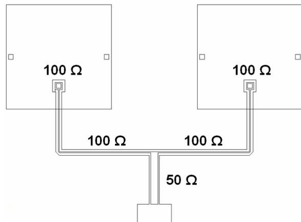
Fig. 4. Design layout of  $2 \times 1$  patch array antenna.
