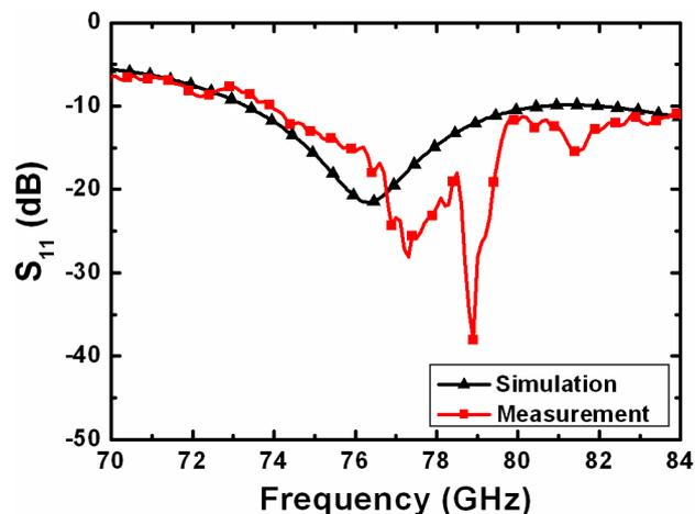
Fig. 9. Simulated and measured results of input return loss for the fabricated  $2 \times 1$  patch array antenna with additional supporting posts.
