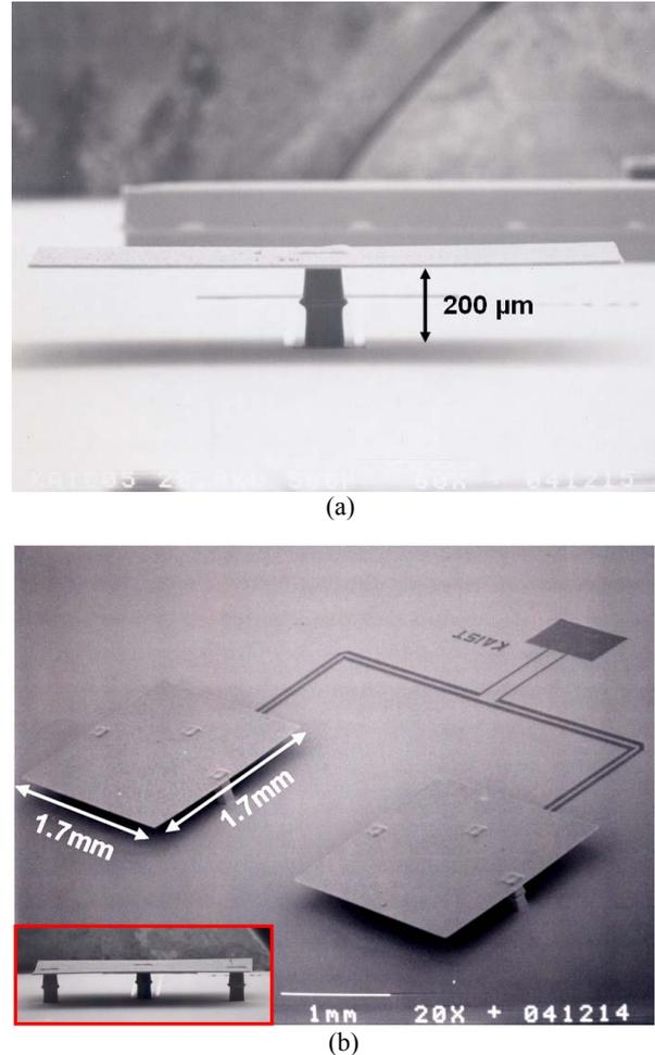
Fig. 6. SEM photographs of the fabricated antenna. (a) The cross sectional view of single patch antenna without additional supporting posts. (b) The perspective view and cross sectional view of  $2 \times 1$  patch array antenna with additional supporting posts.
