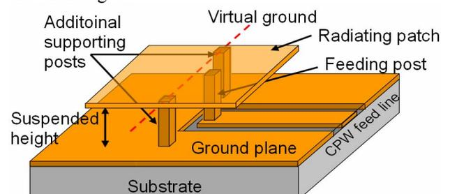
Fig. 1. Illustration of the proposed antenna structure. Additional supporting posts are optional for the robustness.
