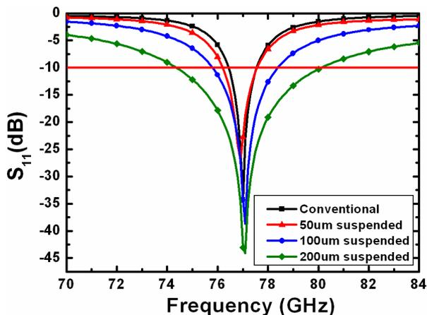
Fig. 3. Simulation result of input return loss for conventional printed patch antenna and proposed antenna with various suspended heights.
