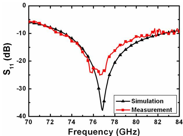
Fig. 8. Simulated and measured results of input return loss for the fabricated single patch antenna with additional supporting posts.
