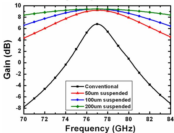
Fig. 2. Simulation result of gain for conventional printed patch antenna and proposed antenna with various suspended heights.
