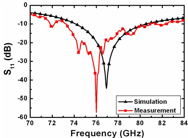
Fig. 7. Simulated and measured results of input return loss for the fabricated single patch antenna without additional supporting posts.
