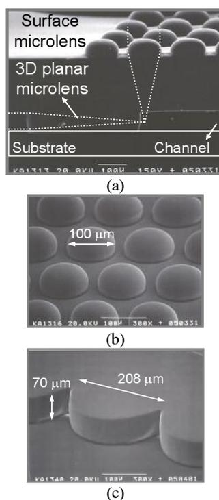
Figure 3. (a) Cross-sectional SEM photograph of the fabricated detection system. The expected paths of lights were also shown with dotted lines. Enlarged photographs of the (b) surface microlens and (c) 3D planar microlens
