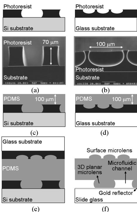
Figure 2. Fabrication process of the integrated optical detection system. (a)(b) Photoresist mold formation by using a 3D diffuser lithography. (c)(d) PDMS spin coating (e) PDMS bonding and curing (f) PDMS peel-off and bonding on a slide glass coated with a gold reflector
