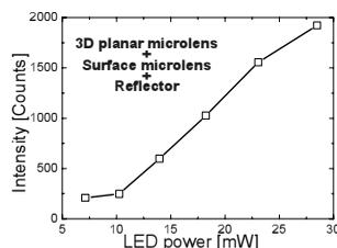
Figure 6. Intensity of the fluorescence light with different powers consumed by LED.
