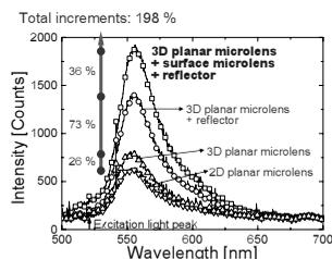
Figure 5. Optical spectrometer measurement results of the fabricated optical detection system with the integrated microlenses and the reflector.
