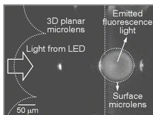
Figure 4. Microscope photograph showing the emitted fluorescence light through the surface microlens when an LED was used for an excitation source
