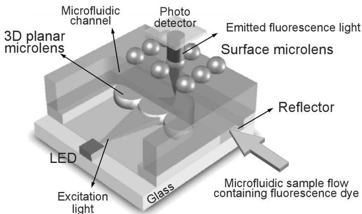
Figure 1. Schematic view of the proposed optical detection system for an extremely low-power and low-cost disposable lab-on-a-chip
