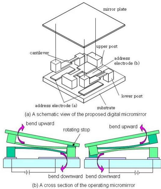
Figure 1. Schematic views of the micromirror device and its operation principle [2]
