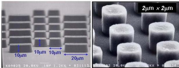
Figure 3. SEM images of various dimensions of electroplated posts
