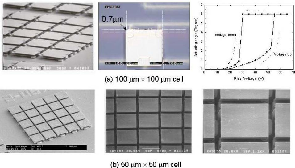
Figure 4. Fabrication results of high fill-factor micromirror arrays
