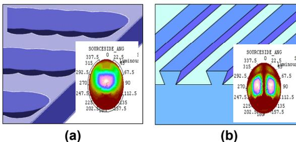
Fig. 1 Shapes of light extraction structures, (a) dumbbell-like (b) bar-like.
