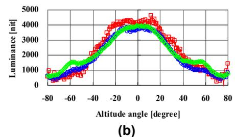
Fig. 4 Optical properties of fabricated LGP sample in the mold frame. The measured luminance value at (a) 0 degrees and (b) 90 degrees at 3 points of LGP (front, center, and rear position from the light sources).
