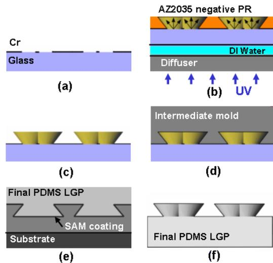
Fig. 2 Fabrication process of the dumbbell-like bump: (a) embedded mask, (b) backside 3D diffuser lithography, (c) photoresist mold after development, (d) replication of intermediate mold, (e) replication of final PDMS LGP, and (f) peeling off the final LGP from the intermediate mold.
