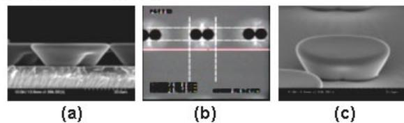
Fig. 3 Images of the fabricated patterns: (a) SEM image of photoresist pattern, (b) top view image of intermediate mold using optical microscope, and (c) SEM image of the final PDMS LGP.
