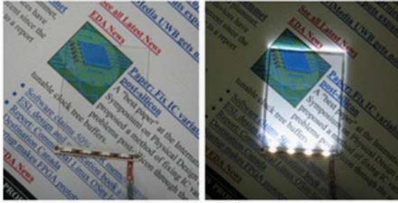
**Fig. 12 A flexible FLU which is just a flipped-over BLU having the inverse-trapezoidal micropatterns**
