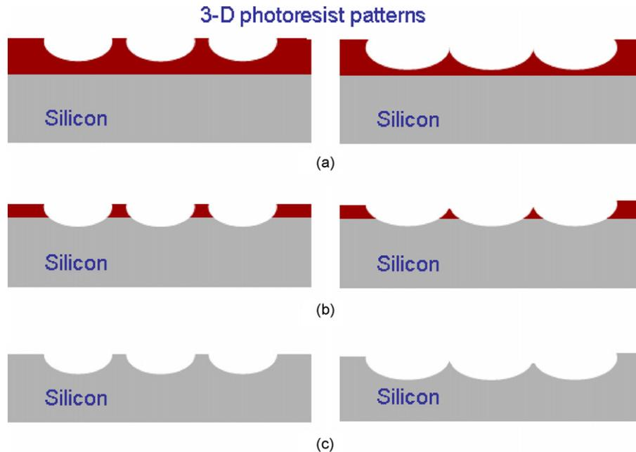
Fig. 3. Process flows of pattern transfer to silicon using ICP etching process: (a) 3-D photoresist patterns on silicon, (b) pattern transfer to silicon during ICP etching process, and (c) 3-D silicon microstructure after ICP etching process.
