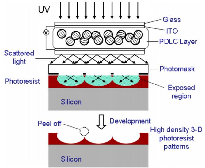
Fig. 2. Schematic views showing the fabrication principles for high density 3-D photoresist microstructures by 3-D lithography using PDLC films.
