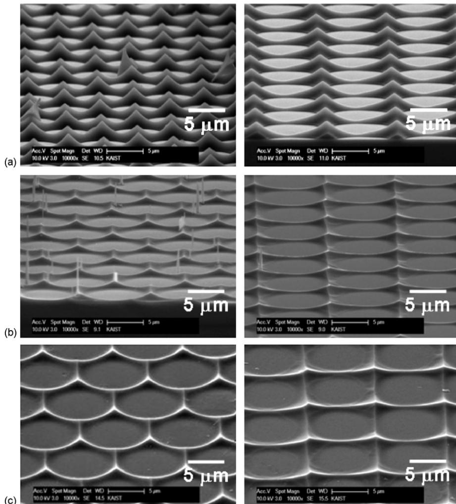
Fig. 5. SEM images of (a) 3-D photoresist microstructures on a silicon substrate by 3-D lithography, (b) 3-D silicon microstructures by ICP etching process, and (c) 3-D silicon microstructures by dipping process with wet-etchant.
