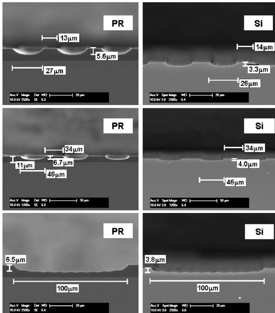
Fig. 4. SEM images of cross-sections of 3-D photoresist microstructures with various sloping profiles acquired by 3-D lithography (left) and 3-D silicon microstructures transferred by ICP etching (right).
