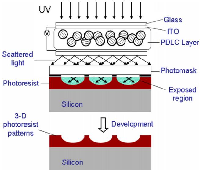
Fig. 1. Schematic views showing the fabrication principles for 3-D photoresist microstructures by 3-D lithography using polymer dispersed liquid crystal (PDLC) films.
