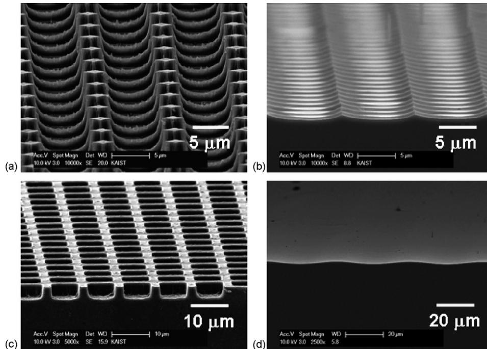
Fig. 6. (a–d) SEM images of various shapes or slopes of 3-D silicon microstructures.
