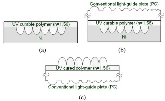
Figure 8. The fabrication process of the designed LGP : the conventional LGP mounting the microlens array.
