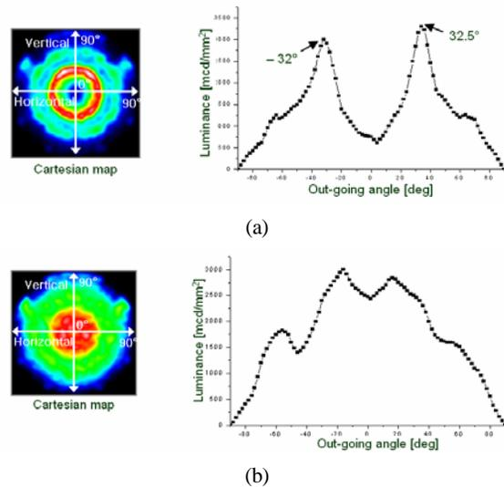
Figure 3. The luminance profiles of the proposed BLU simulated by SPEOS (Optis Co.): (a) the intensity distribution on the designed LGP; (b) the intensity distribution on the designed LGP plus the conical microlens array sheet.
