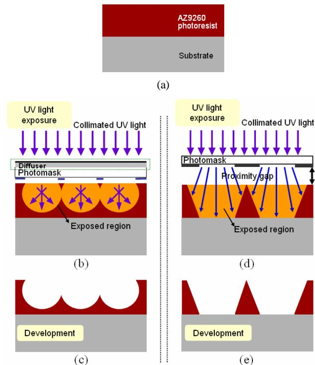
Figure 4. The fabrication process of the microlens array mold and the conical microlens array mold: (a), (b), and (c) for the former; (a), (d), and (e) for the latter.
