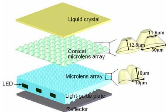
Figure 1. A schematic view of the proposed BLU.
