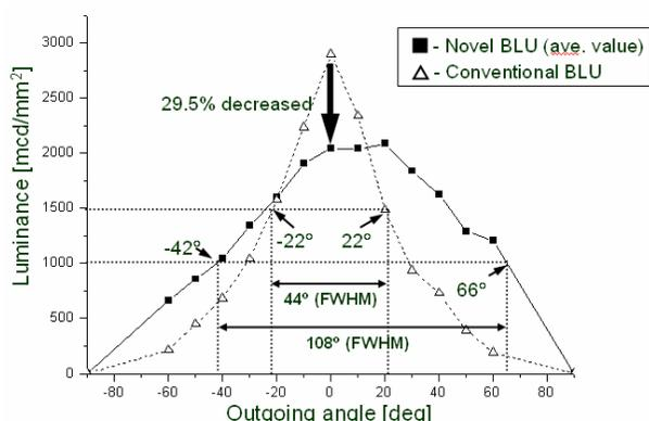
Figure 10. The average luminance distribution of the proposed BLU compared to that of the conventional BLU.
