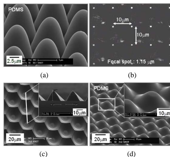
Figure 5. SEM photographs of the microlens array and the conical microlens array : (a) the PDMS replica of the microlens array and (b) the focal spot of it; (c) the photoresist mold of the conical microlens array and (d) the PDMS replica of it.
