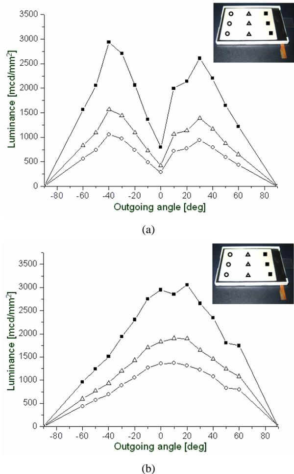
Figure 9. The measured luminance profiles of the proposed BLU : (a) the intensity distribution on the designed LGP only; (b) the intensity distribution on the proposed BLU including the conical microlens array sheet.
