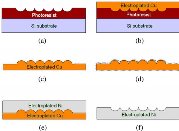
Figure 6. The fabrication process flow chart of Ni-stamper.
