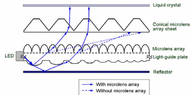
Figure 2. The conceptual ray trajectory in the proposed BLU.
