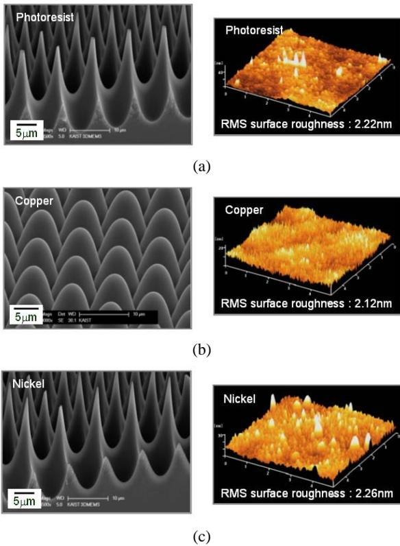
Figure 7. SEM photographs of the each step to fabricate Ni-stamper and their surface roughness measured by AFM.
