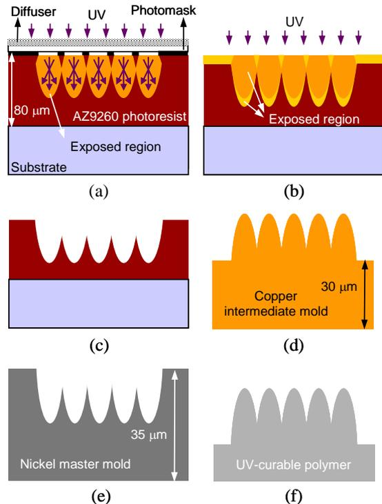
Fig. 1. Fabrication process of an MLA: (a) the 1<sup>st</sup> UV exposure on the photoresist through a diffuser and photomask, (b) the 2<sup>nd</sup> UV flood exposure, (c) fabricated photoresist mold after development, (d) fabrication of a copper intermediate mold and (e) a nickel master mold by electroplating, and (f) plastic replication from the nickel master mold.
