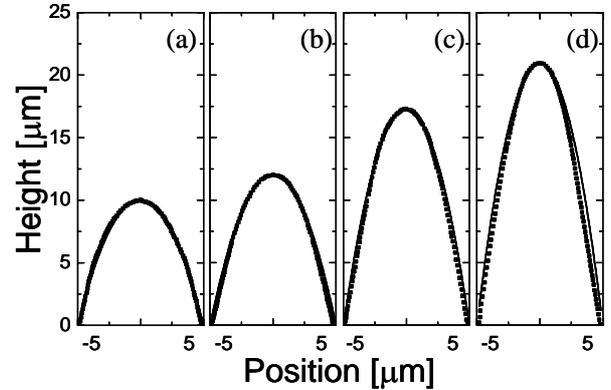
Fig. 3. The actual profile of the fabricated microlens (square dots) and the ideal parabolic profiles (solid lines) with different aspect ratios of (a) 1.0, (b) 1.2, (c) 1.7, and (d) 2.1.
