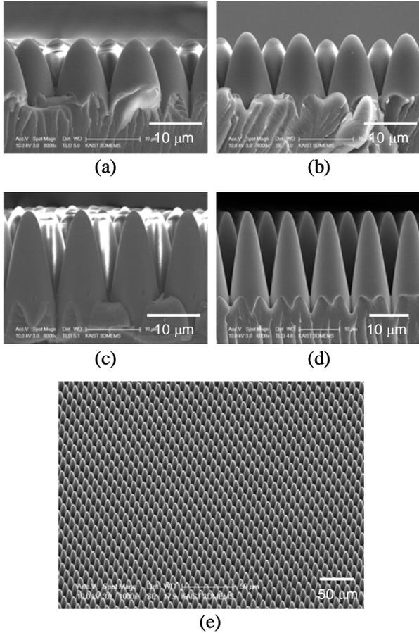
Fig. 2. SEM photographs of the fabricated plastic MLAs with a pitch of 10  $\mu\text{m}$  and various heights of (a) 10  $\mu\text{m}$ , (b) 12  $\mu\text{m}$ , (c) 17  $\mu\text{m}$ , and (d) 21  $\mu\text{m}$ . (e) Bird's eye view of the MLA with a height of 21  $\mu\text{m}$ .
