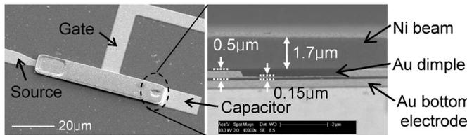
Fig. 3. SEM images of the fabricated microswitch-based MORAM and a magnified view of the air-gap region between the suspended Ni beam and the Au bottom electrode.
