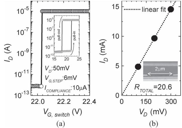
Fig. 4. (a)  $I_D$  versus  $V_{G,switch}$  characteristics. (b)  $I_D$  versus  $V_D$  characteristics showing the total on resistance of the fabricated microswitch.
