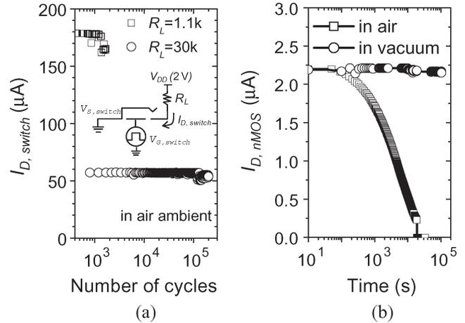
Fig. 6. (a) Endurance and (b) retention characteristics of the fabricated microswitch-based MORAM.
