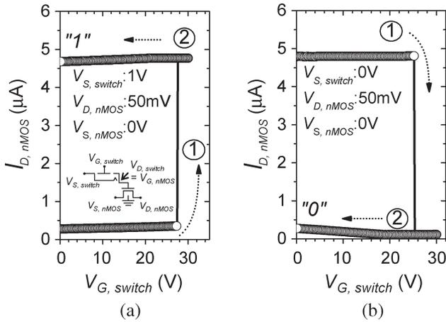
Fig. 5.  $I_{D,nMOS}$  versus  $V_{G,switch}$  for showing the (a) program operation and (b) erase operation of the fabricated MORAM, where the number in the circle shows the sweep sequence of the  $V_{G,switch}$ . The inset shows the experimental setup for characterizing memory operations of the fabricated MORAM.
