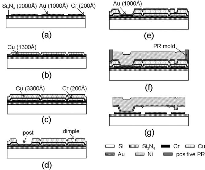
Fig. 2. Simplified fabrication process of the metallic microswitch-based MORAM using a metal surface micromachining technology. (a) Bottom electrode formation. (b) Cu sacrificial deposition. (c) Cr/Cu sacrificial deposition. (d) Dimple and post wet etching. (e) Au deposition for contact. (f) Ni beam plating (1.7  $\mu\text{m}$ ). (g) Sacrificial etching and Ni beam release by CPD.
