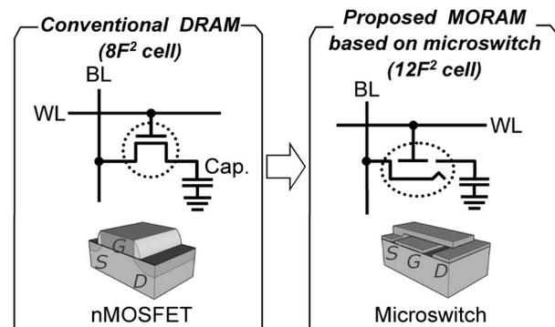
Fig. 1. Schematic diagram and equivalent circuit of the conventional DRAM and the proposed MORAM based on the microswitch, which is similar to the DRAM except that the nMOSFET is replaced with the metallic microswitch.
